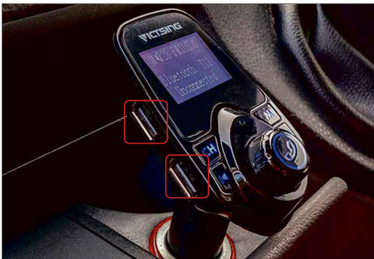
Some FM transmitters, like this VicTsing model, have USB ports for memory sticks and charging devices
