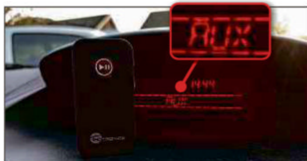
If your car has a 3.5mm jack or phono sockets, you can connect a Bluetooth receiver and use the radio's auxiliary source to play your music
