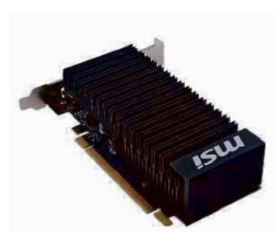
Some graphics cards - like MSI's Nvidia 1030 - are silent, due to metal fins that dissipate heat
